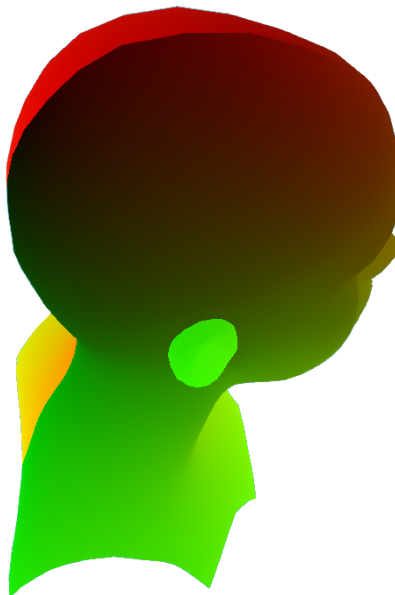
Figure 2.1: Head model with UV-coordinates projected onto it's surface. Visible seams appear at the ears and at the top of the head and down along the neck area.
